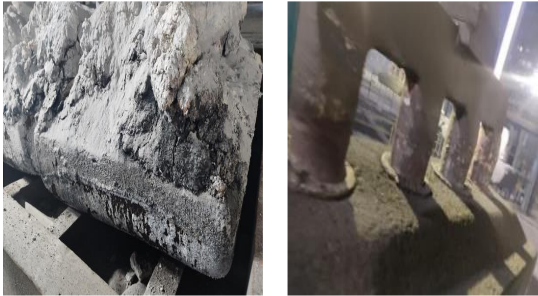
Figure 10. Coated anode butts. Left: Butt Profile, Right: Top oxidation.
