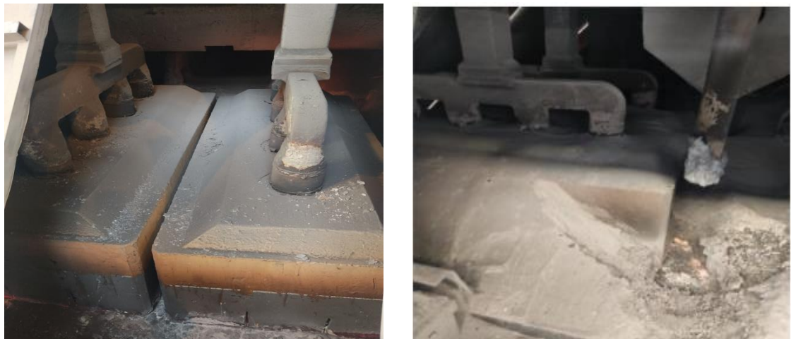
Figure 3. Coated anode sample condition inside pot. Left: After anode change, Right: Tap end.
